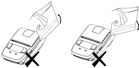
If you insert a card tilted upward/downward into the MSR slot, the card does not move horizontally and a read error occurs.
