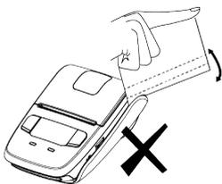
If you insert a card into the middle part of the MSR card, the card is not read correctly and read error occurs, or if you move the card back or forth by force after inserting into the MSR slot, the card is not read correctly and a read error occurs.
