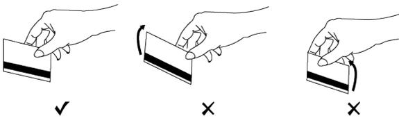
If you grasp the front/rear part of a card and move it through the MSR slot, the front /rear part is loose and a read error occurs.
