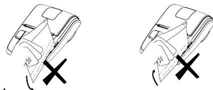
If you extract a card at the end of the MSR slot by lifting up or lowering down, the card is not maintained and a read error occurs.
