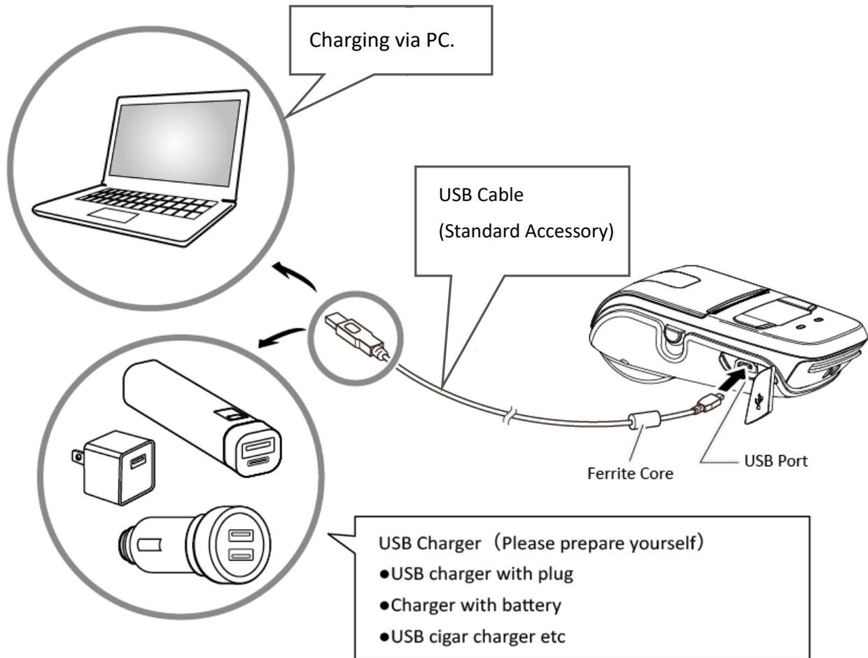
When battery pack runs out of power, the battery icon will flash. It powers off automatically when continues printing. If you want to go on, please charge it.
