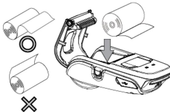
3) Pull the end of the roll straight toward you. Then press down on both sides of the printer cover to close it firmly. When you close the printer cover, make sure that it is closed on both sides.
